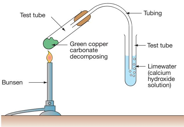
**Figure 3.2** Decomposition of copper carbonate.
