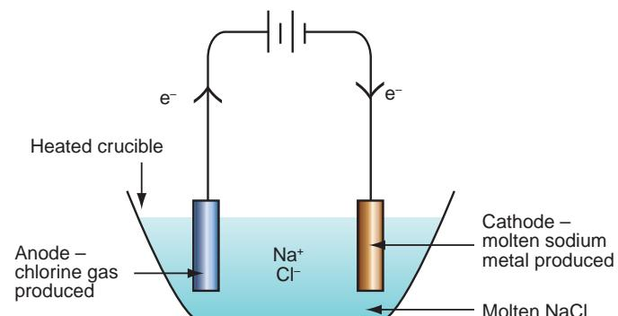
**Figure 3.2** Decomposition of molten sodium chloride by electrolysis.
