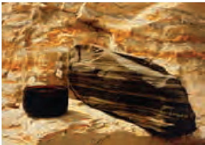
**Figure 5.4** A block of shale oil and beaker of crude oil extracted from this type of rock.
